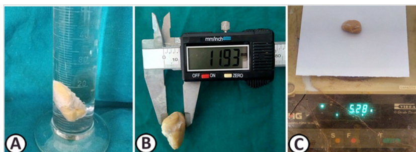
Figure 3. A: A graduated cylinder for measuring the volume of the SGs, B: A digital caliper for measuring of the thickness of the SGs, C: A sensitive scale for measuring of the weight of the SGs.
