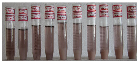
Figure 7. Effect of pH on the photocatalytic degradation of textile effluent at 120 minutes [textile effluent =3%]
