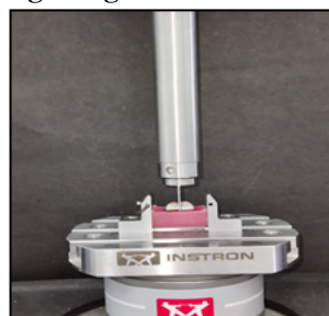
Figure 2. Bond strength testing using INSTRON E 3000 universal testing machine.
