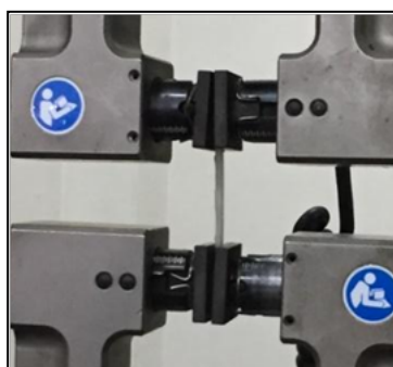
Figure 3. Evaluation of tensile strength in universal testing machine.
