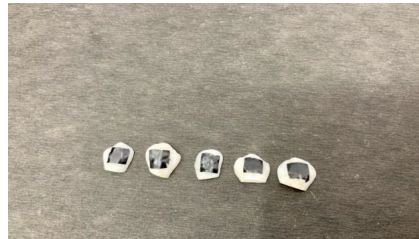
Figure 3. The specimens are mounted on acrylic blocks.
