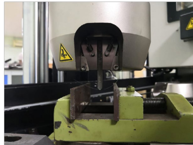
Figure 4. Full deflection of 5mm given.
