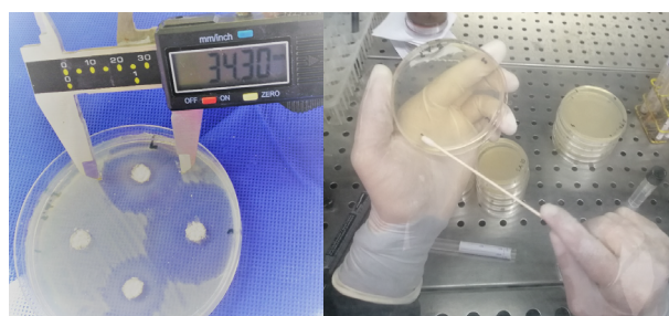
Figure 1: a. b. measure the diameter of inhibition zone by digital caliper.
