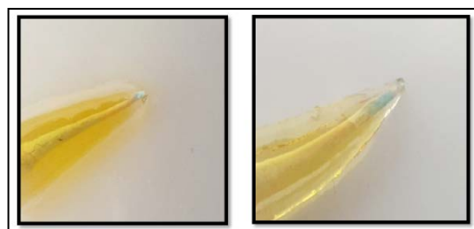
Figure 1. Dye penetration test shows less microleakage in ultrasonic activation sample (left) than sample without activation (right).
